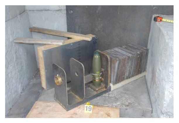
Figure 2: Set-up of the shaped charge jet tests
